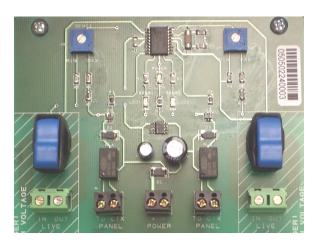
Calibration of the PM2 is easy, once wired set the fan speed controller to setting 1 (or low setting) for example.
